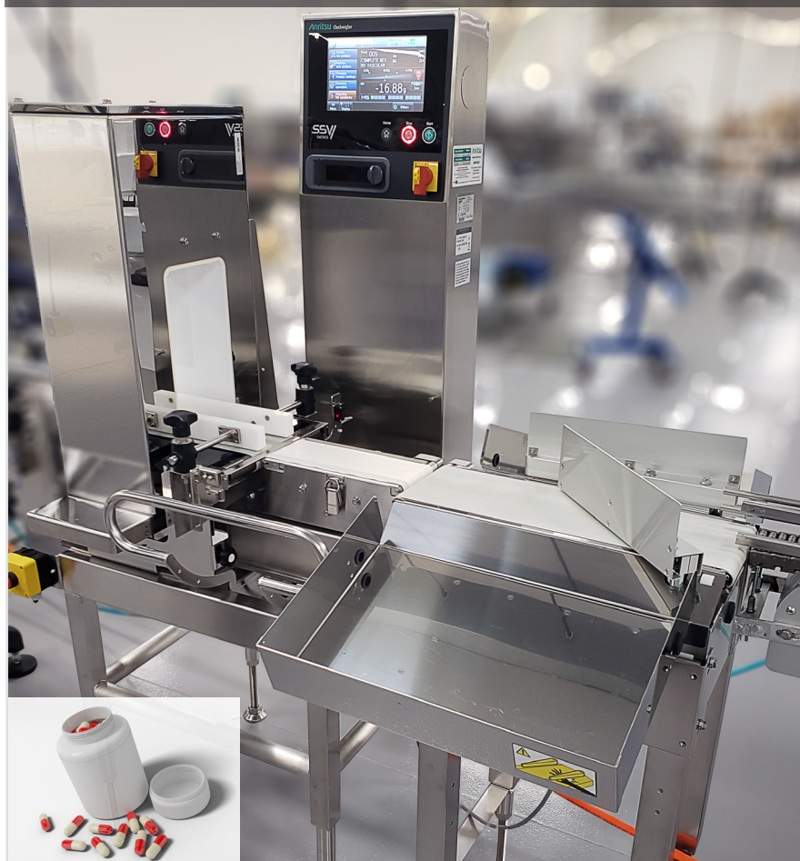
Example installation with vertical metal detector and dual flipper reject
